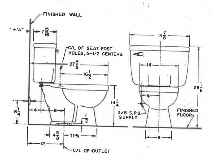
NOTE: 3/8" SUPPLY PIPE NOT INCLUDED WITH FIXTURE AND MUST BE ORDERED SEPARATELY. \*DIMENSIONS SHOWN FOR SUPPLY ARE SUGGESTED.
