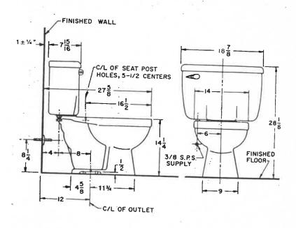
NOTE: 3/8" SUPPLY PIPE NOT INCLUDED WITH FIXTURE AND MUST BE ORDERED SEPARATELY. \*DIMENSIONS SHOWN FOR SUPPLY ARE SUGGESTED.
